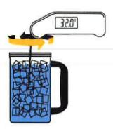
affect your reading. Keep the probe tip away from the side walls and don't allow it to rest against the bottom of the vessel. Doing so will give you inaccurate temperature readings. If the thermometer has an extremely fast and sensitive needle tip, like the Thermapen, you MUST gently stir the probe or you will find colder and warmer spots in the ice bath. Stirring equilibrates the temperature throughout the vessel.
