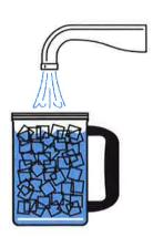
below the top of the ice. Let the mixture sit for a minute or two to allow the temperature of the water to settle. If you see the ice starting to float off the bottom of the vessel, pour off some water and add more ice. Water below the ice will not be at 32°F.
