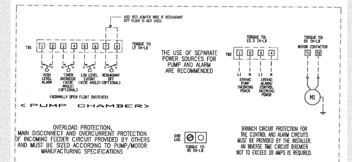
TEMPERATURE RATING OF FIELD INSTALLED CONDUCTORS MUST BE AT LEAST 140 DEG. F. (60 DEG. C.). TERMINAL STRIPS AND GROUND LUG USE COPPER CONDUCTORS ONLY.
