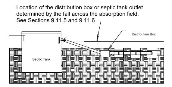
Note: Capping material must extend 10 ft. from trenches before the start of the slope. The tapered slope shall be 3:1 or less.
