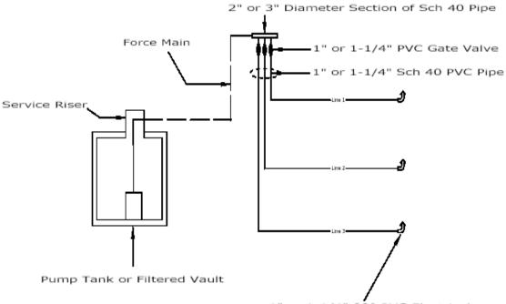
1" or 1-1/4" 90° PVC Electrical Sweep with Ball Valve or Plug
